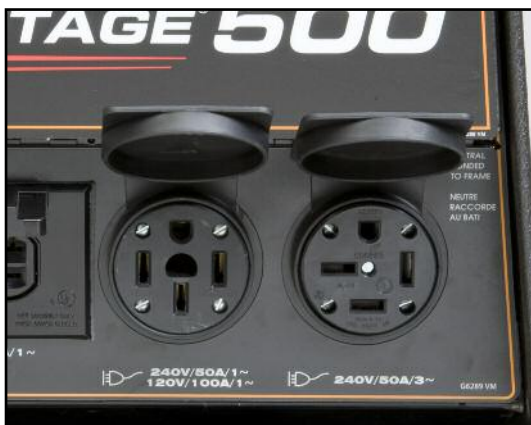
240V 1-Phase and 3-Phase Receptacles with Covers
