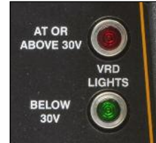
VRD™ portion of nameplate with green light on.
